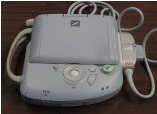
Fig. 4 A compact, portable ultrasound system was used for the echocardiographic evaluations in the high Arctic. The unit was battery-powered to allow unencumbered scanning in the field
