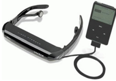
Fig. 3 A virtual guidance system was created using currently available technology (an iPod and 3D video glasses, iWear IP230, Vuzix Corp, Rochester, NY, USA) to allow an ultrasound operator to view a procedural video while performing an ultrasound examination
