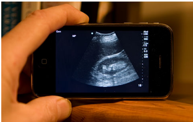
Fig. 2 An example of an image (right upper quadrant Morrison’s Pouch) transmitted to an iPhone
